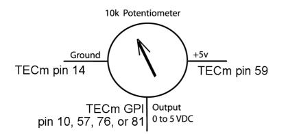
Potentiometer wiring for Fuel, Ignition and GPO Trim Inputs
