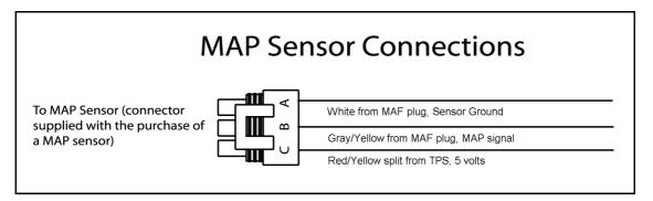
The MAP sensor should then be connected to the intake manifold where it can receive a solid representative pressure reading of the pressure at the intake ports. On the stock manifold, the sensor can be connected to
