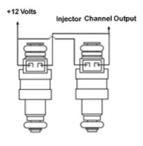
Figure: Parallel wiring of fuel injectors.
